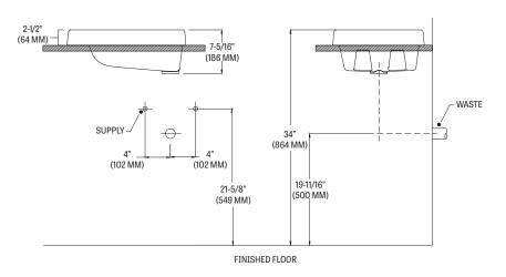
Fixture performance and specifications meet or exceed ASME A112.19.2-2013/CSA B45.1-13 standards, and other state and local codes.
