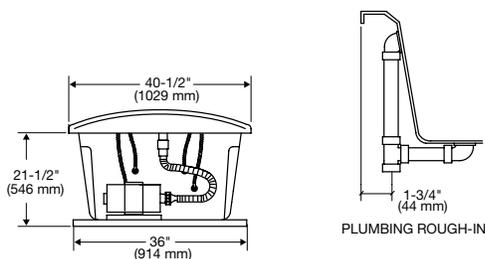
INSTALLER NOTE: DUE TO THE FREEFORM SHAPE OF THIS TUB IT IS RECOMMENDED THAT THE TUB BE ON THE JOBSITE BEFORE MAKING THE FINAL CUT OUT FOR DROP IN INSTALLATION.
