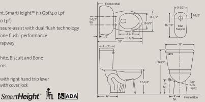
\*NOTE: Install this product according to the installation guide. Fixture dimensions are nominal and conform to tolerances in ASME Standard A112.19.2-2008/CSA B45.1-08.
