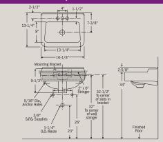
\*NOTE: Install this product according to the installation guide. Fixture dimensions are nominal and conform to tolerances in ASME Standard A112.19.2-2008/CSA B45.1-08.
