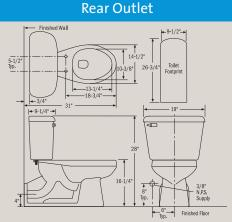
\*NOTE: Install this product according to the installation guide. Fixture dimensions are nominal and conform to tolerances in ASME Standard A112.19.2-2008/CSA B45.1-08.
