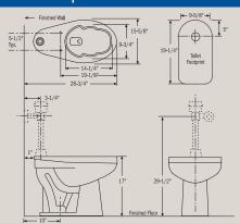
\*NOTE: Install this product according to the installation guide. Fixture dimensions are nominal and conform to tolerances in ASME Standard A112.19.2-2008/CSA B45.1-08.
