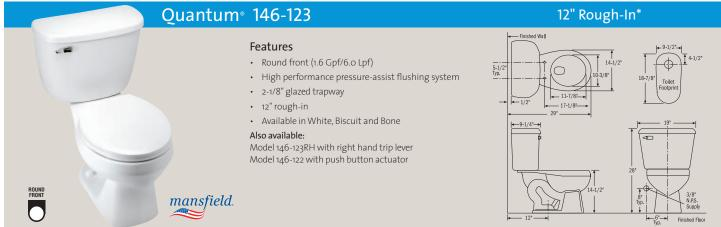
\*NOTE: Install this product according to the installation guide. Fixture dimensions are nominal and conform to tolerances in ASME Standard A112.19.2-2008/CSA B45.1-08.
