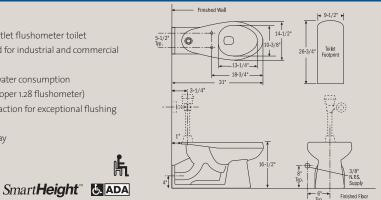
\*NOTE: Install this product according to the installation guide. Fixture dimensions are nominal and conform to tolerances in ASME Standard A112.19.2-2008/CSA 845.1-08.
