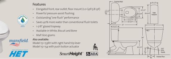
\*NOTE: Install this product according to the installation guide. Fixture dimensions are nominal and conform to tolerances in ASME Standard A112.19.2-2008/CSA B45.1-08.
