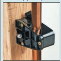
The new Main Block<sup>TM</sup> 1<sup>1</sup>/2" offset pipe clamp is designed with 3-axis holding power and rigidly secures <sup>3</sup>/<sub>4</sub>" to 1" CTS water main inlets, appliance and fixture stub outs, water heater and softener loops. The twopiece pipe clamp is a non-corrosive and 100% compatible with copper, PEX, PVC and CPVC. It installs quickly and is packaged with all installation hardware. Creates a solid connection that ensures a uniform, professional look every time and
