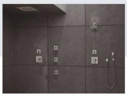
Toto's Legato Shower System features a contemporary squared showerhead, handshower and controls. The Overhead Rain Shower with EcoPower Lighting System includes an LED lighting system that is powered by the flowing water. Shape Memory Alloy valves prevent drastic water temperature changes or scalding. Gyrostream body sprays include nozzles oriented on two different axes that tilt and rotate. Circle No. 161 on Product Card
