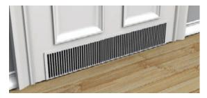
Air-Flow Enhancer. When you need to increase air movement between rooms, the *Perfect Balance In-Door Pressure Balancer* offers a more elegant solution than leaving an enormous gap beneath the door. The 24-inch-by-4-inch grille is made of high-impact ABS plastic and features an interior baffle to reduce noise and light transmission. Though it's made only in white, it can be painted to match any color scheme, says the maker. Prices are \$30 for one unit, \$80 for a three-pack.
