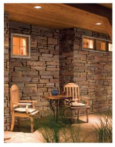
Lightweight Stone. Although BellaStone looks remarkably authentic — thanks to the real stone used in the manufacturing process — the 50-inch-by-24-inch panels weigh a fifth as much as traditional stone and install 50 percent faster, says the maker. The panels have sound-deadening properties and an R-value of at least 2.5, and are sold in three color blends. Installed costs average \$12 per square foot.
