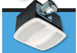
**Air King.** The AKF100D Deluxe Quiet dual-speed exhaust fan fulfills whole-house ventilation requirements with two speeds. Energy Star qualified and California Title 24 compliant, the unit includes a 26-watt fluorescent lamp and a 4-watt night light that can be wired separately. The fan operates at 0.3 sone on the low setting and 1.5 sones when running at 100 cfm. 877.304.3785. www.airkinglimited.com. Circle 186.
