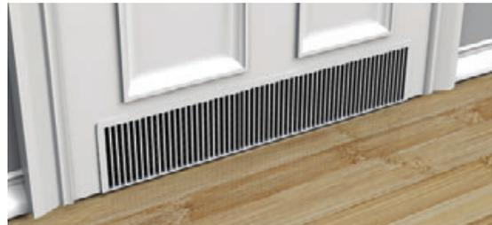
**Air-Flow Enhancer.** When you need to increase air movement between rooms, the *Perfect Balance In-Door Pressure Balancer* offers a more elegant solution than leaving an enormous gap beneath the door. The 24-inch-by-4-inch grille is made of high-impact ABS plastic and features an interior baffle to reduce noise and light transmission. Though it's made only in white, it can be painted to match any color scheme, says the maker. Prices are \$30 for one unit, \$80 for a three-pack.
